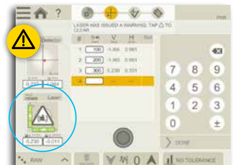
The built-in sensors warns on the display on events which can affect the measurement reliability.
